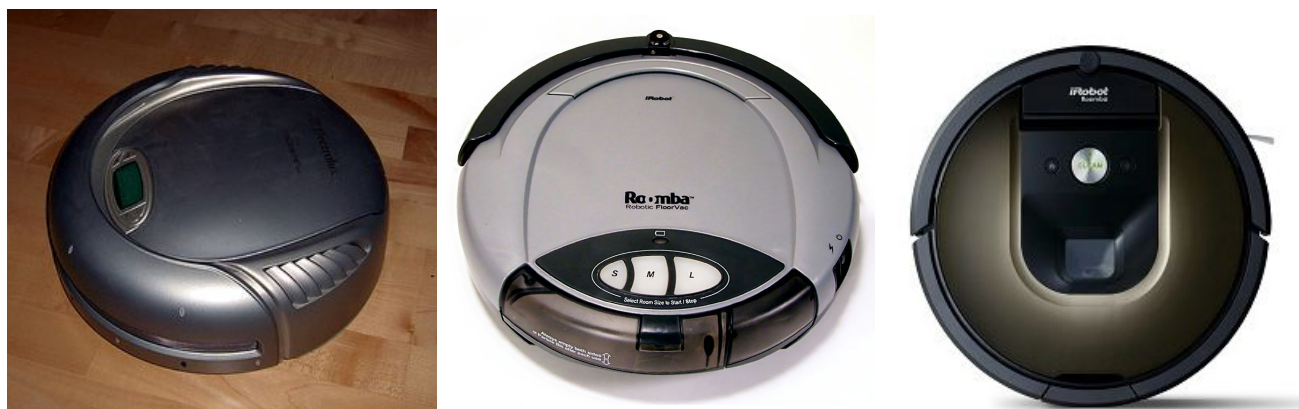
Fig 5.1.2-1: (from left) Electrolux Trilobite (1997), iRobot Roomba (2002) and iRobot Roomba (2015), showing a fairly mature external design. Despite price decreases and functionality improvements, there is still room for incremental improvement.
